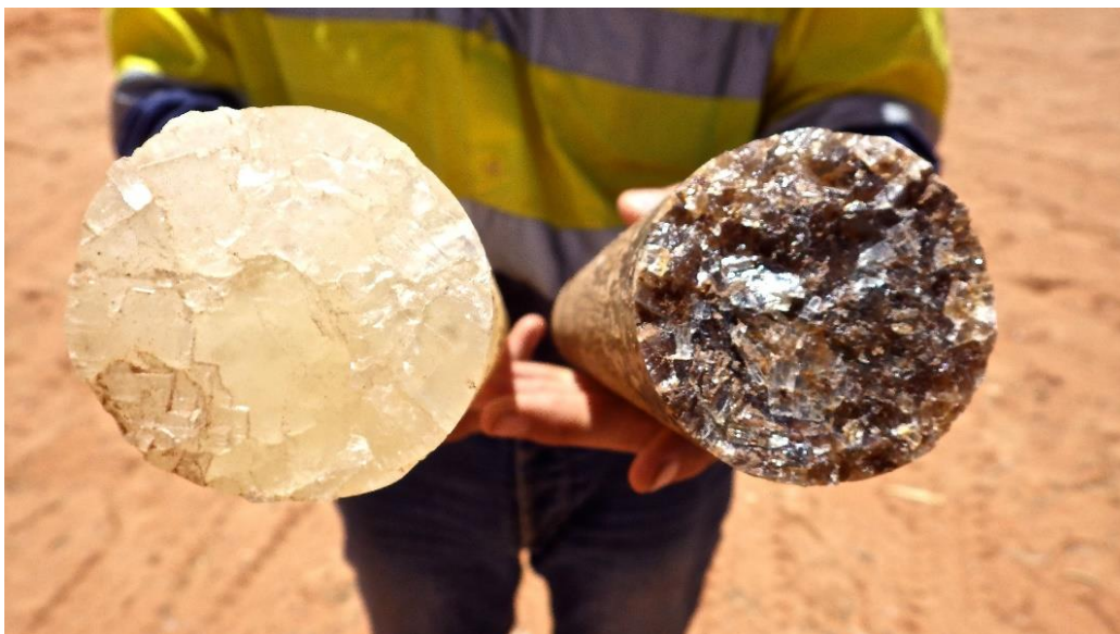
Fig 3: Pure salt core on left and salt core with associated minerals on the right
