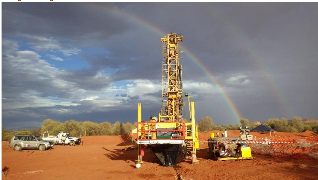
Fig 1: Drilling salt core at CH003
